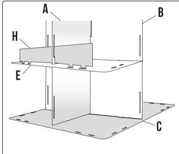
STEP 6: Fit all acrylic boards H through slids in boards A and B and snap into boards E and F.
