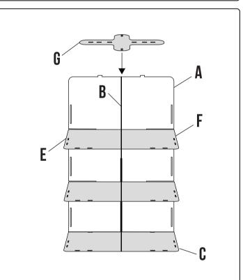
**STEP 5**: Fit all shelves (E + F) into board  $\bf A$  and connect board  $\bf G$  to the top center of  $\bf A$  and  $\bf B$ .
