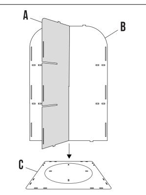
**STEP 2**: Connect the cross wall (A+B) to the bottom board **C**.
