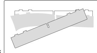
Remove the film from both sides of the acrylic boards **H**. **TIP:** Rubbing 2 of the films against each other will help lift the film.
