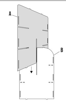
**STEP 1**: Fit slots of boards **A** into board **B** creating the cross walls for the center.
