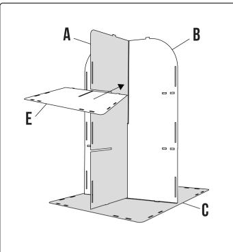
STEP 3: Insert board E to interlock with board A.
