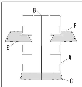
**STEP 4**: Board **F** goes opposite of board **E** when inserting to interlock to board **A**.
