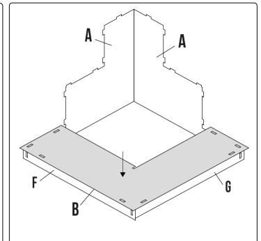
STEP 2: Connect shelf B to the bottom front and back boards F, G and the 2 A boards.
