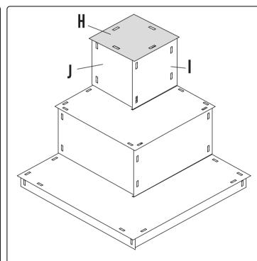
STEP 6: Connect top board H to boards I, J and both boards A.
