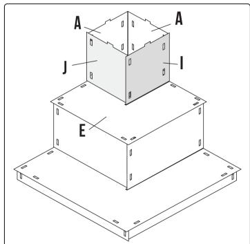
**STEP 5**: Slide board I into board E. Connect board J to board I. Connect both boards to the sides of boards A.
