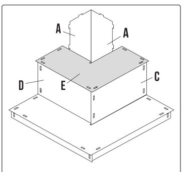
STEP 4: Connect board E to the boards C, D and the 2 A boards.
