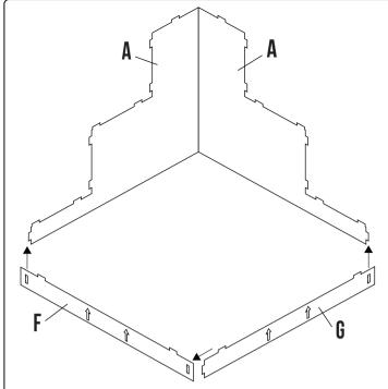
STEP 1: Fit board **G** into board **F** creating the front v-shape bottom of the stand. Connect **F** and **G** to the 2 **A** boards completing the bottom of the stand.
