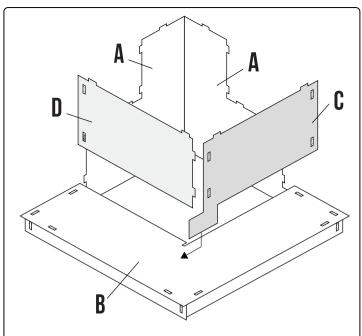
STEP 3: Insert board  $\boldsymbol{C}$  under board  $\boldsymbol{B}$  at the middle of the shelf and connect it to board  $\boldsymbol{A}$ . Insert board  $\boldsymbol{D}$  into board  $\boldsymbol{C}$  and board  $\boldsymbol{A}$ .
